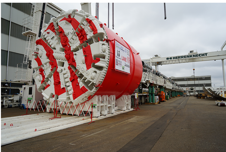
Figure 12: MudHoney, the 18 foot diameter Tunnel Boring Machine, will build the conveyance tunnel for the Ship Canal Project. (Image from: https://spushipcanal.participate.online/ , accessed December 29, 2022.)
